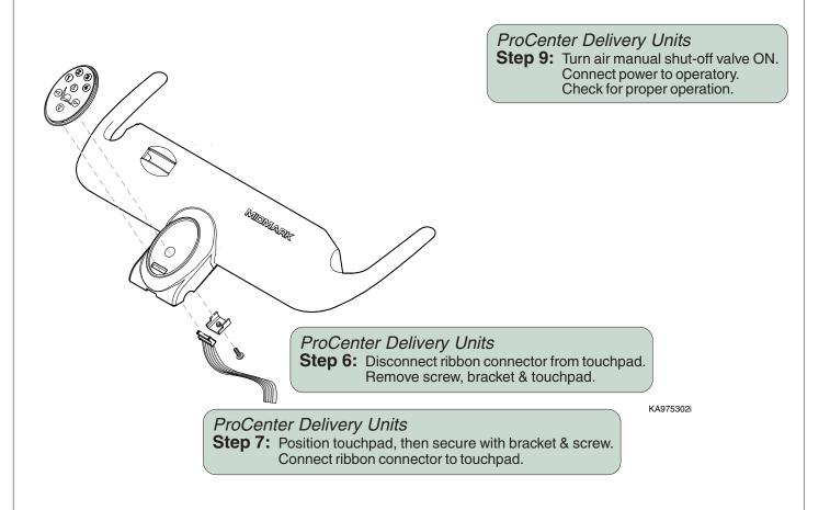
**Step 8:** Position master switch & front cover. Secure cover with eight screws.
